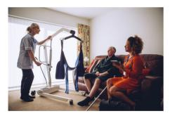
A **hoist** is an electrical piece of equipment that can either help a person move from a seated into a standing position (standing hoist), or a larger hoist can be used to move a person that is unable to stand from one place to another. A hoist can be mobile (on wheels so that it can be moved) or fixed (attached permanently, to a frame or the ceiling), depending on what is most suitable for the person and environment.
